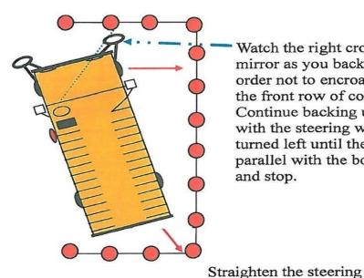
Watch the right crossover mirror as you back up in order not to encroach on the front row of cones. Continue backing up with the steering wheel turned left until the bus is parallel with the box line and stop.
