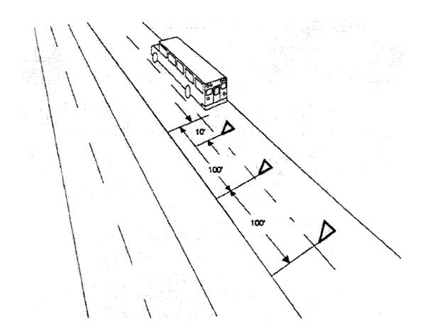
When placing the triangles, hold an assembled triangle <u>toward</u> the oncoming traffic. This enhances safety by increasing visibility to other drivers (especially at night).
