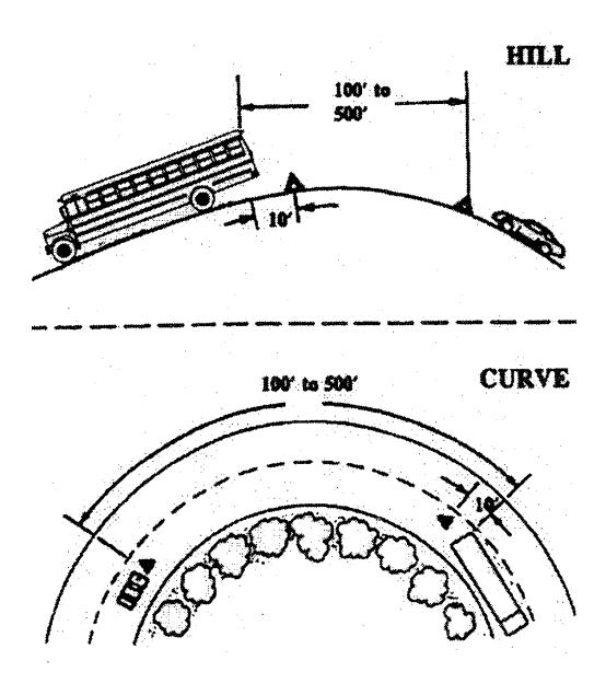
Reminder: If the line of sight is obstructed due to a hill or curve, move the rearmost triangle to a point giving adequate warning.
