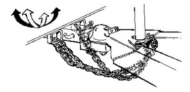
The ball should be located so the trailer sits level when connected to the tow vehicle. The vehicle should be able to accept this weight without a major change of attitude.
