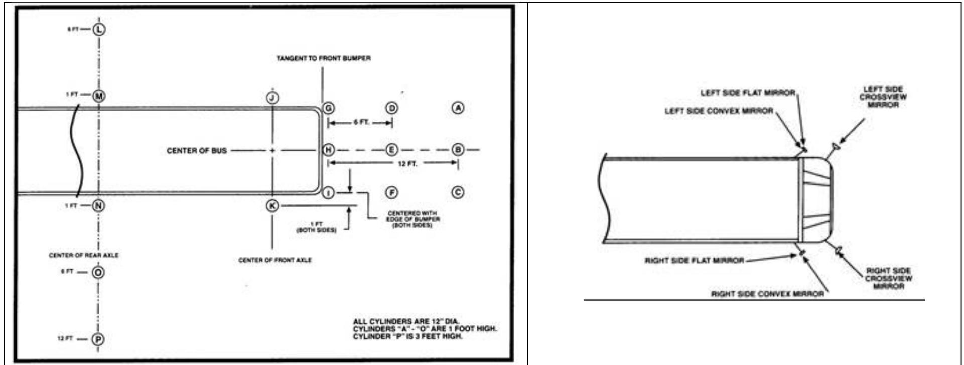
**REAR VIEW MIRRORS (SYSTEM A)** Used together, left side flat mirror and left side convex mirror must provide a view of "M" and, continuing from there, 200 feet rearward of the mirror surface. Used together, right side flat mirror and right side convex mirror must provide a view of cylinder "N" and, continuing from there, 200 feet rearward of the mirror surface.
