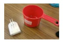
We placed a device called a level indicator in the measuring cup. This makes a chime or vibration when liquid hits a certain level in the measuring cup. The student was alerted to touch the roll n' pour again, which would make it stop pouring.
