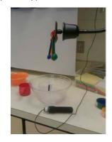
This picture shows a measuring spoon hooked up to the pourer. Here the grasp switch, seen in the bottom center of the picture, is used. Squeezing it would signal the pourer to turn the measuring spoon,
